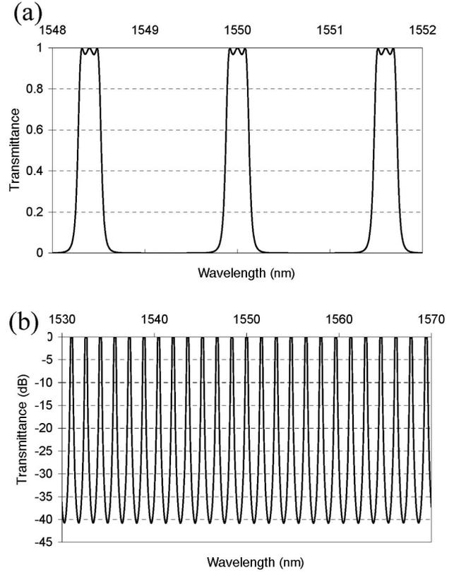
Fig. 5. Theoretical transmission spectrum of the interleaver: (a) linear scale and (b) decibel scale. The structure design is as follows: HLH/246L<sub>2</sub>/HLH/A/, HLH/246L<sub>2</sub>/HLH/A/, and HLH/246L<sub>2</sub>/HLH, with  $n_H = 2.09$ ,  $n_L = 1.46$ ,  $n_{L2} = 1.444$ ,  $n_A = 1$ . External medium air.
