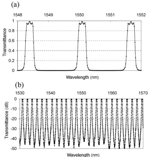
Fig. 7. Experimental transmission spectra of the interleaver: (a) linear scale and (b) decibel scale. The structure design is as follows: HLH/1864 $L_2$ /HLH/air; HLH/1864 $L_2$ /HLH/air; and HLH/1864 $L_2$ /HLH; where H, Ta<sub>2</sub>O<sub>5</sub>; L, SiO<sub>2</sub>;  $L_2$ , silica substrate; external medium air.
