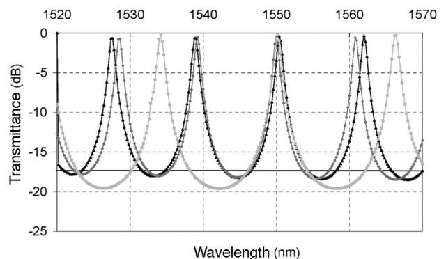
Fig. 3. Experimental transmission spectra of the three single SSFs. The structure designs are as follows: Light gray curve,  $(\text{HL})^3\text{H}/186.01 \text{L}_2/(\text{HL})^3\text{H}$  (SSF1); black curve,  $(\text{HL})^3\text{H}/260.02 \text{L}_2/(\text{HL})^3/1.46\text{H}$  (SSF2); gray curve,  $(\text{HL})^3\text{H}/278.03 \text{L}_2/(\text{HL})^3/1.46\text{H}$  (SSF3); where H,  $\text{Ta}_2\text{O}_5$ ; L,  $\text{SiO}_2$ ;  $\text{L}_2$ , silica substrate; external medium, air.
