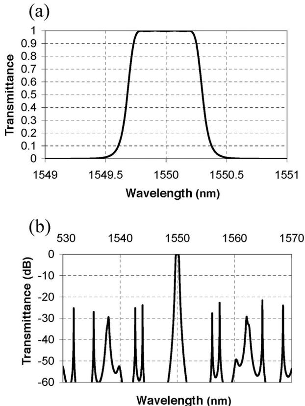
Fig. 1. Four-cavity SSF design following DWDM requirements: (a) linear scale and (b) decibel scale. The structure design is as follows:  $1.09H/(LH)^2/246L_2/(HL)^2/1.05H/20.66A/$ ;  $1.13H/(LH)^2/500L_2/(HL)^2/1.09H/24.79A/$ ;  $1.06H/(LH)^2/412L_2/(HL)^2/1.02H/31.11A/$ ; and  $0.73H/(LH)^2/298L_2/(HL)^2/1.27H/$ , with  $n_H = 2.09$ ,  $n_L = 1.46$ ,  $n_{L2} = 1.44$ ,  $n_A = 1$ . External medium air ( $n_A = 1$ ).
