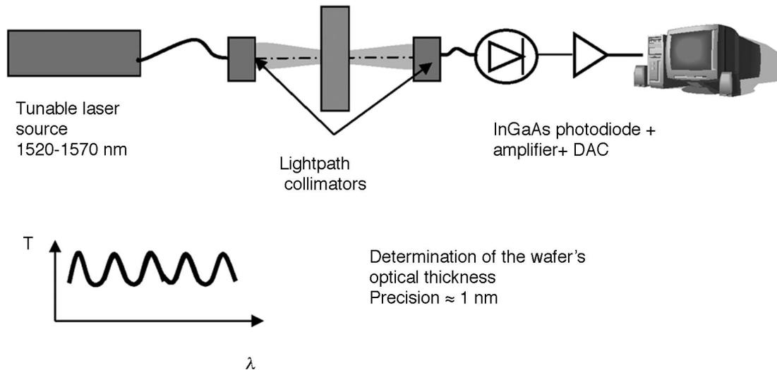
Fig. 2. Principle of measurement of wafer thickness.
